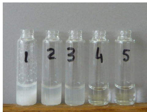
Fig. 5. Direct visual observation of \text{CaCl}_2 /CDP-20-150a mixtures at \text{pH } 9 ( \text{Ca}^{2+}:\text{P}=2.8 , CDP-20-150a at 50, 25, 16.6, 12.5 and 8.3 \text{ g L}^{-1} for tube 1–5, respectively).
